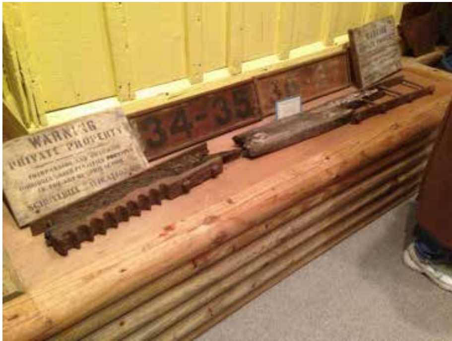
Figures 8 a&b. Lock Wicket Lifting and Lowering Mechanisms
