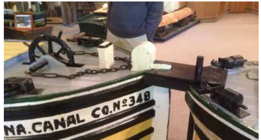
Figure 7. Sectional Boat Steering Mechanism (not properly rigged)
