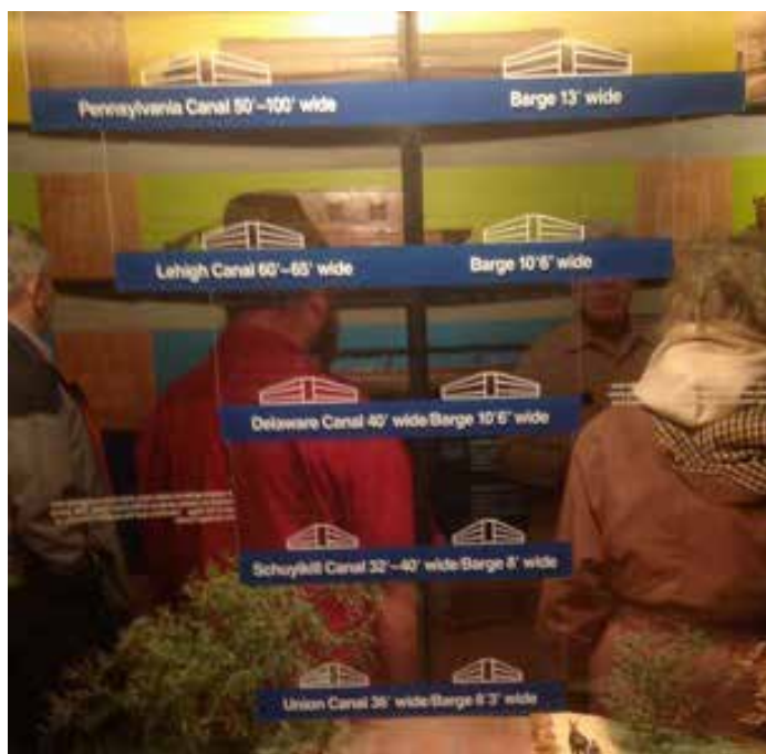
Figure 12. Graphic Showing the Size of Pennsylvania’s Coal Canals and the Boats Employed on Them
